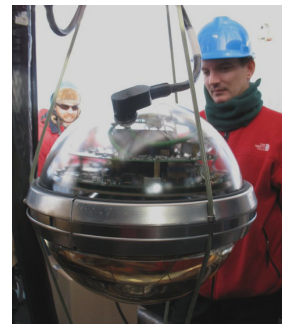
Digital Optical Modules (DOMs) detect signals generated by neutrino collisions in the ice.
